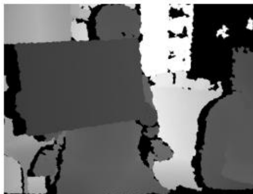
Figure 3. Kinect sensor depth image. Depth sensor from the infrared (IR) point in Figure 2 [3]
