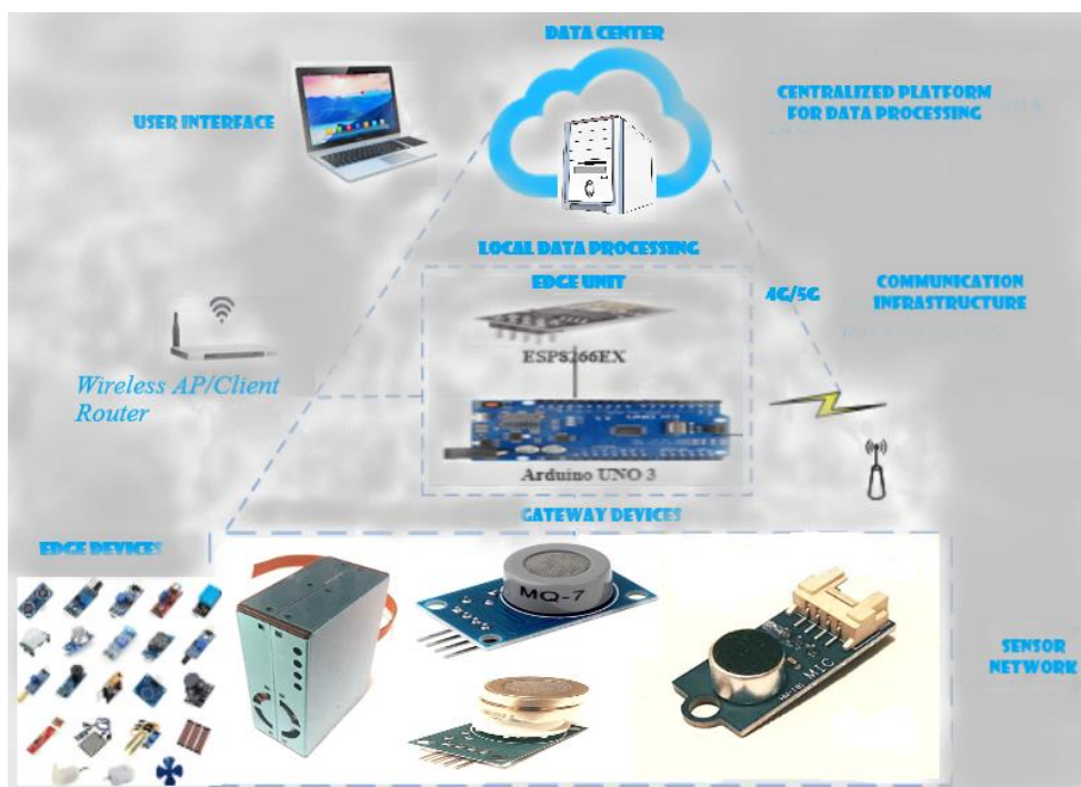
Figure 1: Architecture of the Edge computing system for the formation of the Air Pollution Data Center
