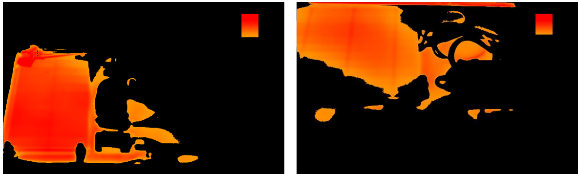
Figure 2. The result of the range between 60°C and 70.5°C shown in the form of a colored mask.
